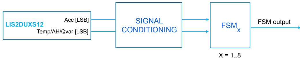
Figure 11. State machine in the LIS2DUXS12
